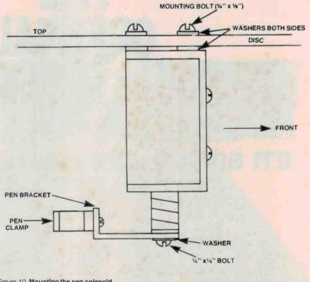
Figure 10. Mounting the pen solenoid.
