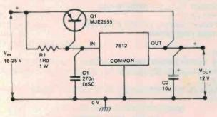
Figure 17. Increasing the output current capacity of a three-terminal regulator. This will deliver 5 A at 12 V.
