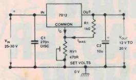
Figure 15. Improved method of varying output voltage.
