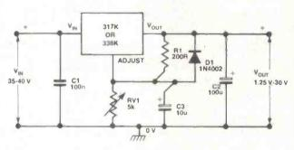
Figure 20. This version of the variable-voltage regulator provides some 80 dB of ripple rejection.
