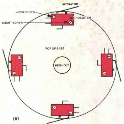
Figure 8. Locating and mounting the mlcroswitches for the 'touch' or 'bump' sensor ring. (a) Orlent the actuators clockwise around the base. (b) The 1" long screw is passed up from under the base through the outermost mounting hole. The %" screw passes downwards through the innermost hole. Use washers under each screw head and nut.
