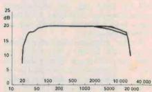
Figure 6. Frequency response of the same head with the same tape types after 3000 hours' use. Note that the frequency response with ordinary oxide tape commences rolling off in the 2 kHz
