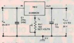
Figure 14. Simple method to vary output voltage.
