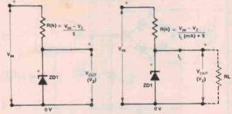
Figure 7. Basic zener reference circuit. Bias is about 5 mA.
