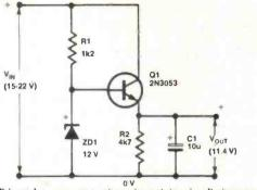
Figure 9. This series-pass, zener-based regulator circuit gives an output of 11.4 V and can supply load currents up to about 100 mA.
