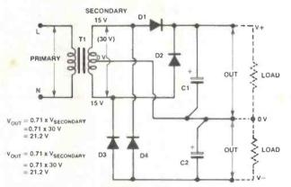
Figure 4. Basic dual supply using individual diodes.
