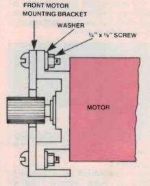
Figure 7. Securing the front face of the motor to the mounting bracket.
