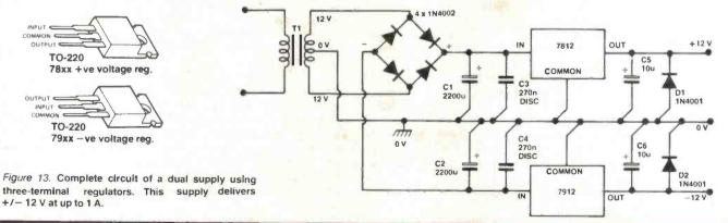
Three-terminal regulators are remarkably easy to use, as shown in the basic circuits of Figures 11 to 13, which show the connections for making positive, negative and dual regulator circuits respectively. The ICs shown in these examples are 12 volt units with current ratings of 1 A, but the basic circuits are valid for all other voltage ratings, provided that the unregulated input voltage is at least three volts greater than the desired output voltage.
