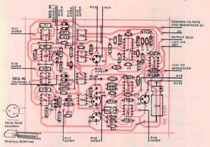
Component overlay. Note that the board has been laid out for the Q1 and Q3 translators with an e-c-b pinout. Watch the pinout of the transistors you use; you may have to cross the base and collector leads.
