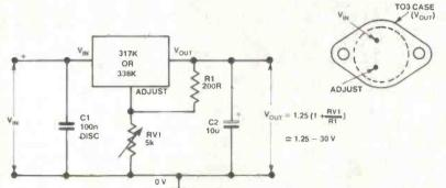
Figure 19. Case outline, basic data and basic application circuit of the 317K and 338K variable-voltage three-terminal regulators.
