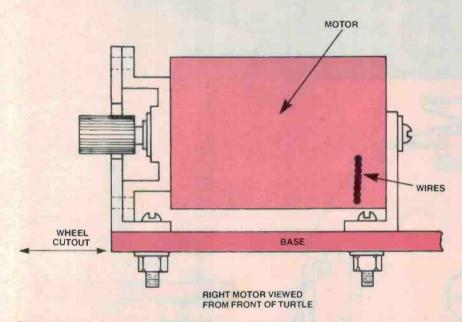
Figure 6. Mounting the motor. Secure the end bracket screw first.
