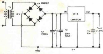
Figure 12. Circult using a common three-terminal negative regulator.
