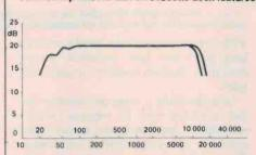
Figure 5. Frequency response of JVC SA head with iron oxide and with chrome tape. Chrome tape has extended frequency response.
