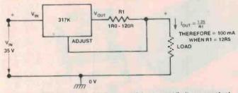
Figure 24. A method of using the 317K as a precision current limiter or constant current generator
