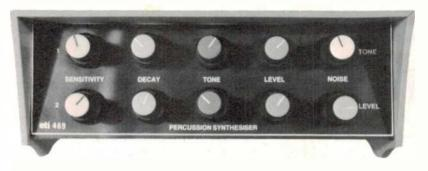
We housed our project in a light but sturdy ABS plastic case and attached a Scotchcal label to the front panel — artwork for this panel is reproduced on page 126. The two 'transducer' inputs, the output and supply input are located on the rear panel. Small speakers serve as input transducers and are mounted in separate small boxes.
