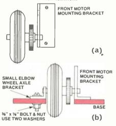
Figure 4. Mounting the wheel assembly to the left hand front motor bracket. (a) Insert the nylon gear end of the axie in the appropriate hole in the front motor bracket (view looking down). (b) Support the other end of the axie with the small axie elbow bracket and temporarily bolt it in place. The right hand wheel assembly mounts in a similar way.
