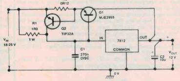
Figure 18. Providing overload protection for the Figure 17 circuit. Q2 'robs' Q1 of base current when load current goes above 5 A.
