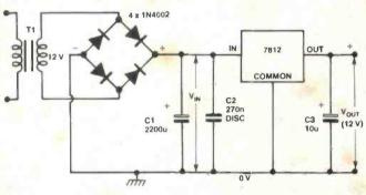
Figure 11. Circuit employing a common three-terminal positive regulator.
