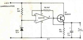
Figure 10. Op-amp based reg. provides 12 V at up to 100 mA with excellent regulation.
